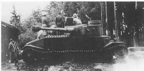
The VK4501(P), or Porsche Tiger, mounted the same Krupp turret with its 88mm gun as the rival Henschel design, but this was positioned further forward than in the Henschel tank, making the Porsche design front-heavy. In this view the turret has been traversed so that the gun faces towards the rear.
