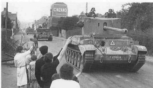
The first British attempt to mount the existing 17-pounder gun in a tank produced the A30 Challenger, based on the Cromwell chassis. This view shows a 2nd Northants Yeomanry tank in Normandy on 17 August 1944. The Challenger was an unsatisfactory expedient that suffered from inadequate levels of armour protection. [IWM B9331]
