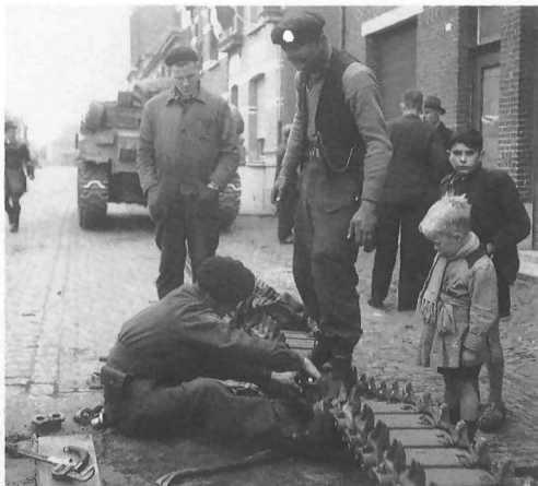
Two of the crew of a Fort Garry Horse Sherman – Corporal R. Young (left) and Sgt G.E. Murray (right) – repair damage to one of the tank's tracks. (PA-137140)
