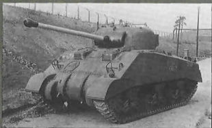
This photograph shows the first prototype Firefly, chassis T148350, which was fitted with a wooden mock-up 17-pounder gun. This photograph was taken in early January 1944 at Chertsey in Surrey. (TfM 2995/B/3)
